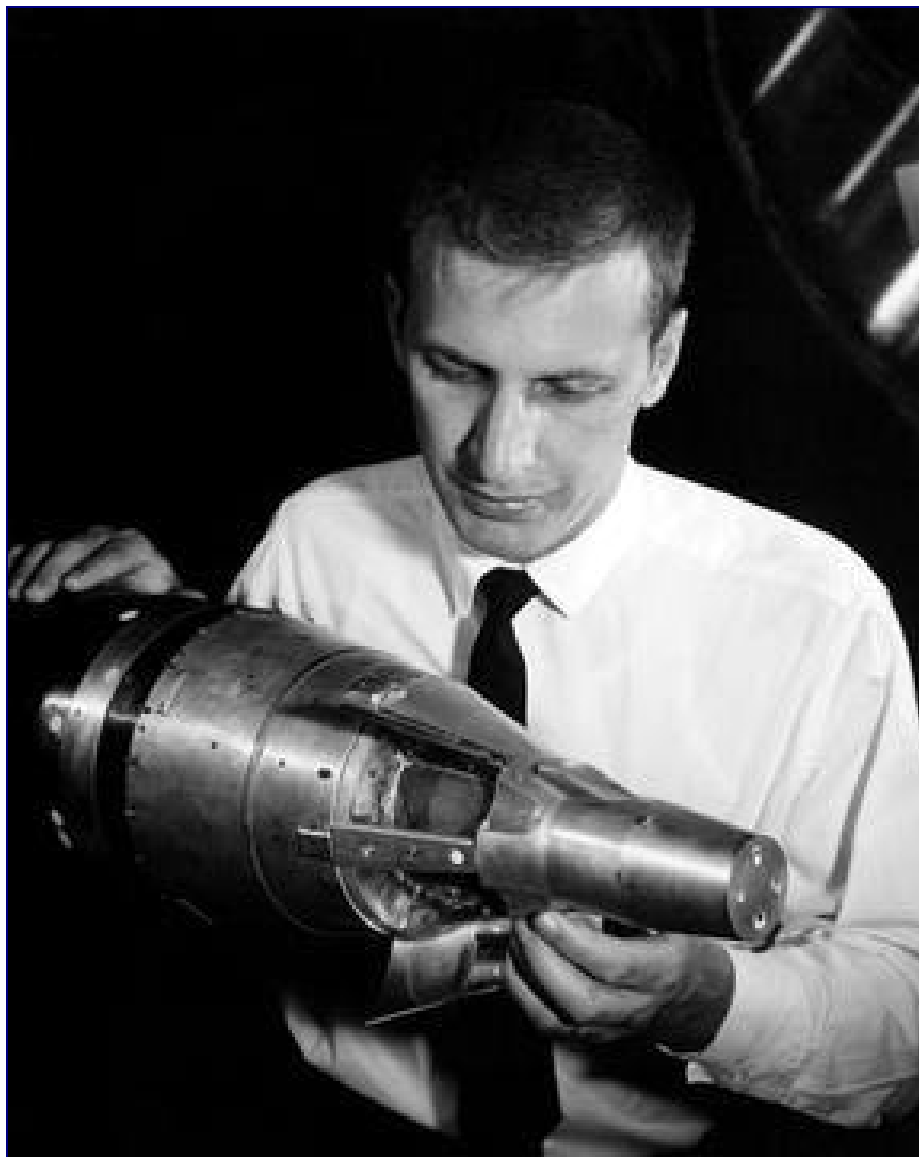
Preparing Gemini Spacecraft Model for Early Wind Tunnel Testing, photo courtesy of NASA.
