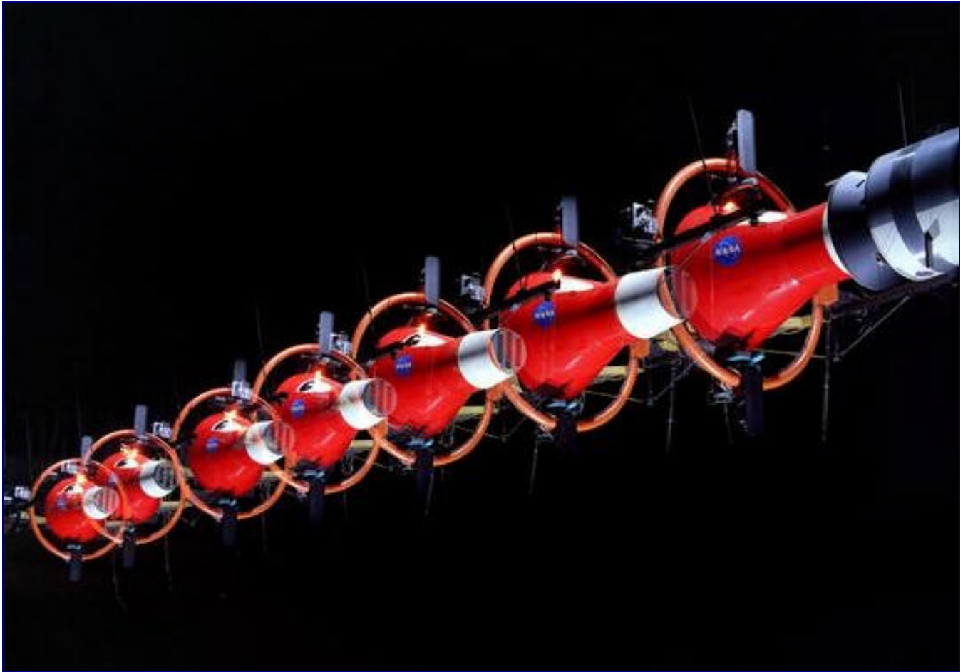
Multiple Photographic Exposure of Rendezvous Technique to be Used for the Spacecraft and Gemini Agena Hard Docking, photo by NASA.
